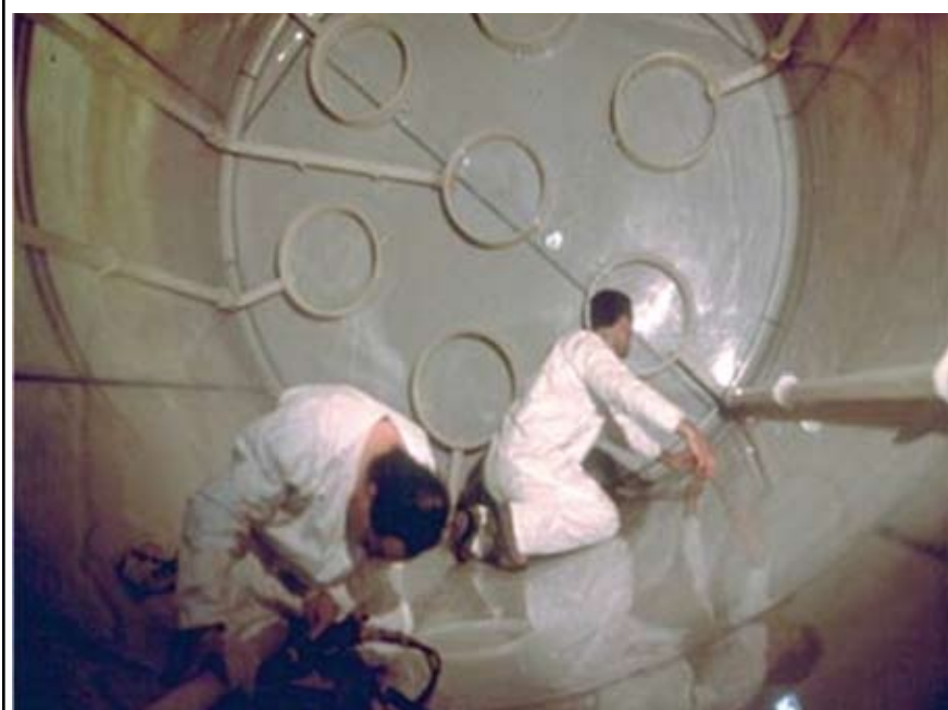
Figure 4. Vessel made from a welded PVDF sheet,
