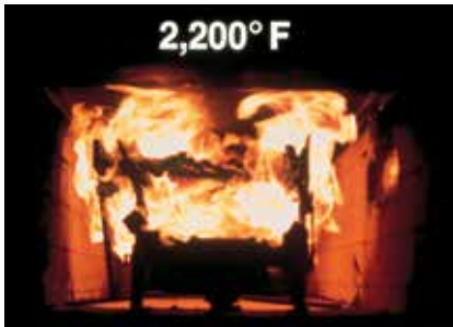
Steiner Tunnel used for ASTM E-84 Testing
