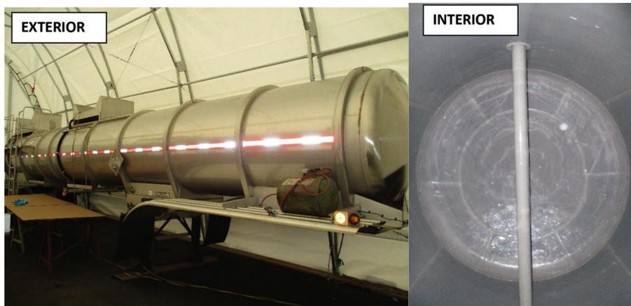
**FIGURE 4** Over-the-road trailers carrying aggressive chemicals can be lined with PVDF copolymers. (Images courtesy of Electro Chemical Engineering & Manufacturing.)
