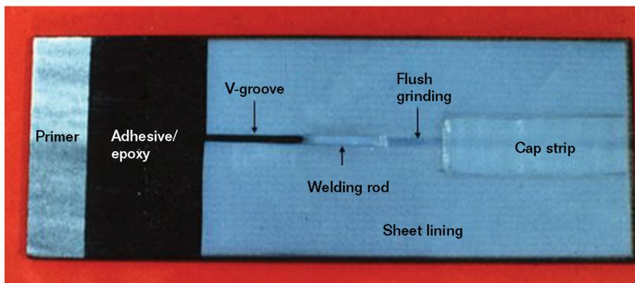
**FIGURE 2** Tank-lining steps. Image courtesy of Electro Chemical Engineering & Manufacturing.
