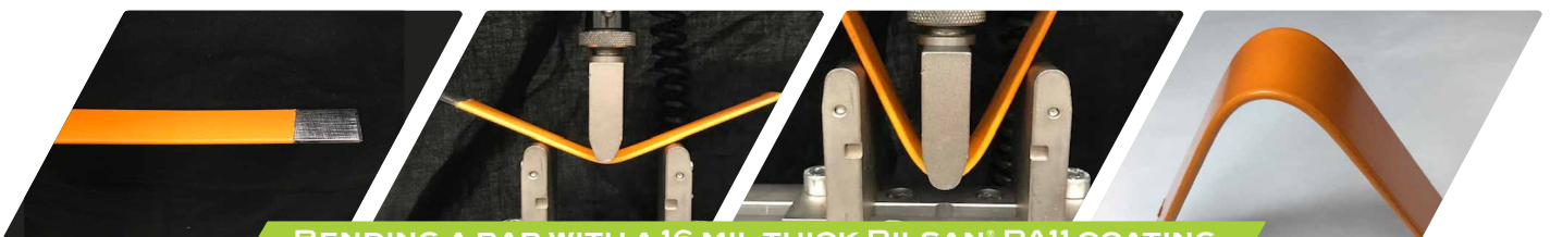
BENDING A BAR WITH A 16 MIL THICK RILSAN ® PA11 COATING
