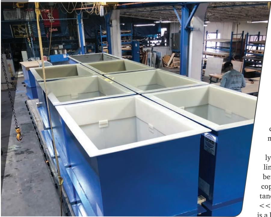
PVDF can outperform its competition by providing longer lasting and trouble-free containment for the most aggressive plating solutions, even at elevated temperatures.
