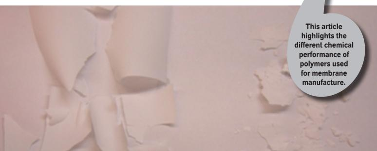
Figure 1: Nylon (PA 6,6) Membrane after Exposure to Chlorine and Sodium Hypochlorite
