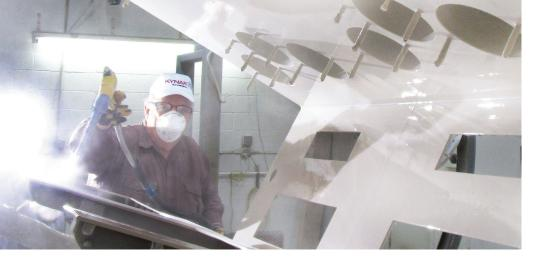
Figure 5. Application of electrostatically sprayed PVDF powder coatings in Graphic courtesy of Fisher Company
