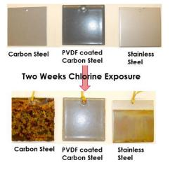
Figure 4. Kynar Flex PVDF coatings versus metal in two weeks of chlorine exposure for Graphic courtesy of Arkema
